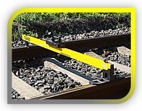
A change from previous versions is the integration of a new control unit equipped with a more powerful CPU and LCD display. Built-in program includes all the necessary tasks for measuring geometrical parameters of tracks (gauge and cant), operating sensor calibration and method of wireless communication with a total station. Measured values of gauge and cant are stored in the internal memory of the TG-03 with data transfer to a PC via USB memory.
